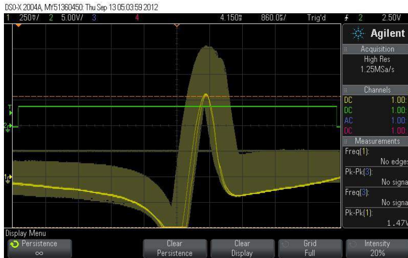
Figure 2.23: Long Term Oscillations Due to the 60 Hz Field
