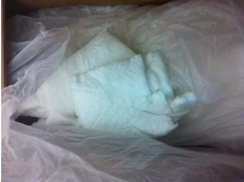
Figure 2.4: Wet Moldable Insulation Sheets
