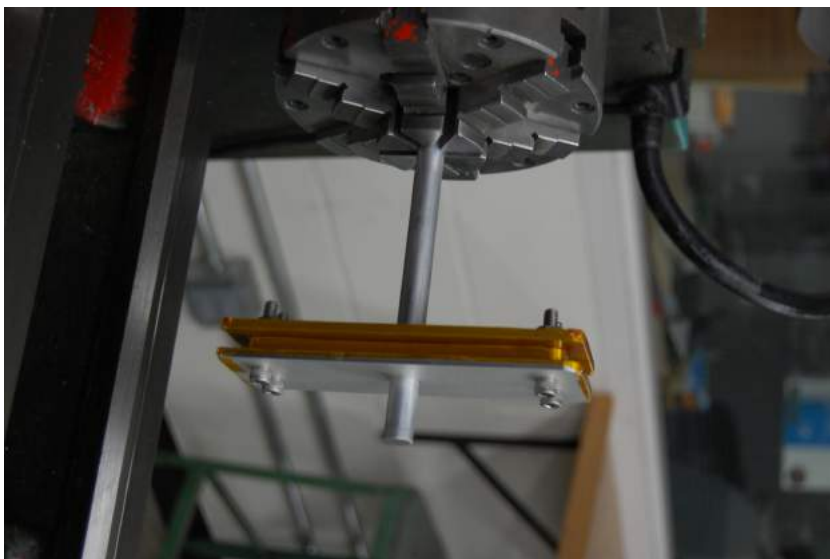
Figure 3.12: A Coil Mount on an Axel, Ready to be Wound Upon
