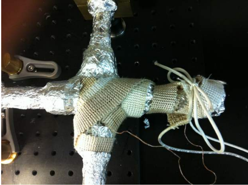
Figure 2.3: Heat Tape Wrapped Around the Pipe for Baking
